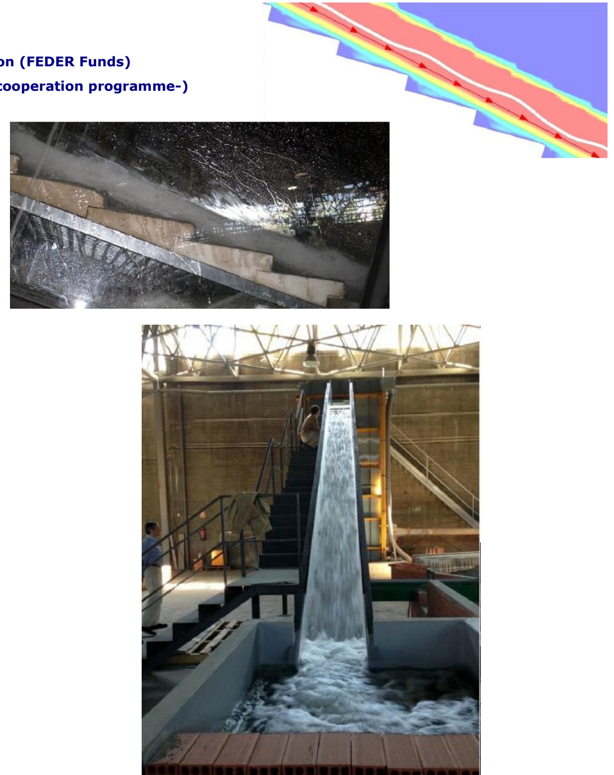
Physical and numerical models of spillway with wedge-shaped blocks.
