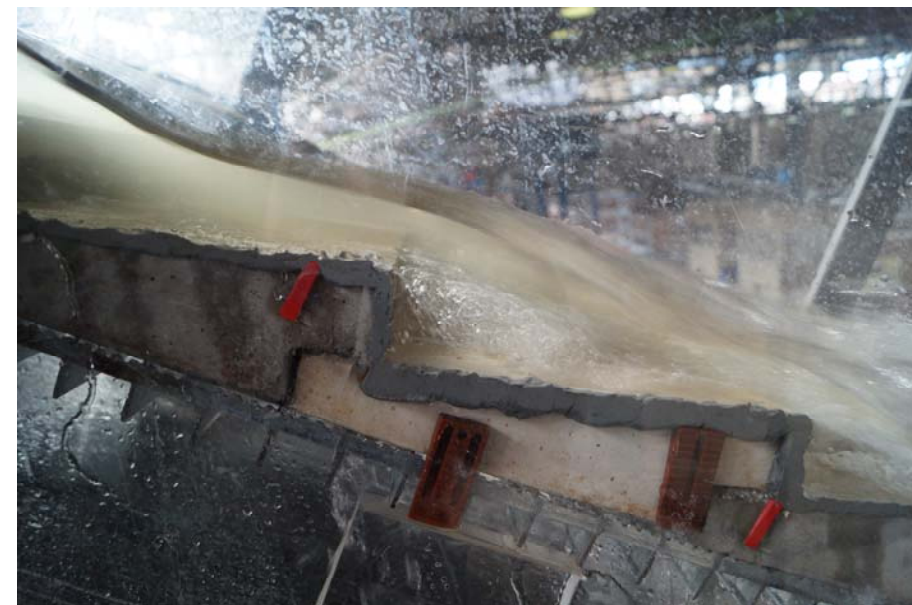
Testing facilities of spillway physical model with wedge-shaped blocks in operation.
