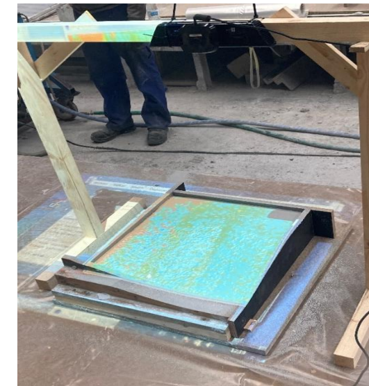
GRC panel sprayed onto a 3D-printed mold with thickness calibration control
