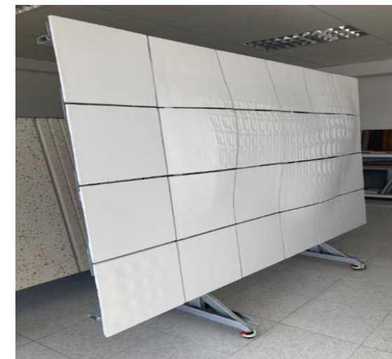
Mock-up with GRC panels
